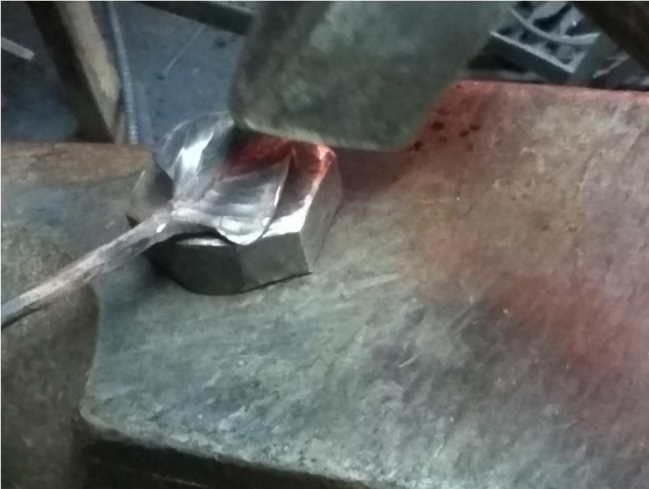
This is a close up of using the cross peen of the hammer to texture the leaf. This is on top of a large bolt that I have forged to fit the hardy hole.
