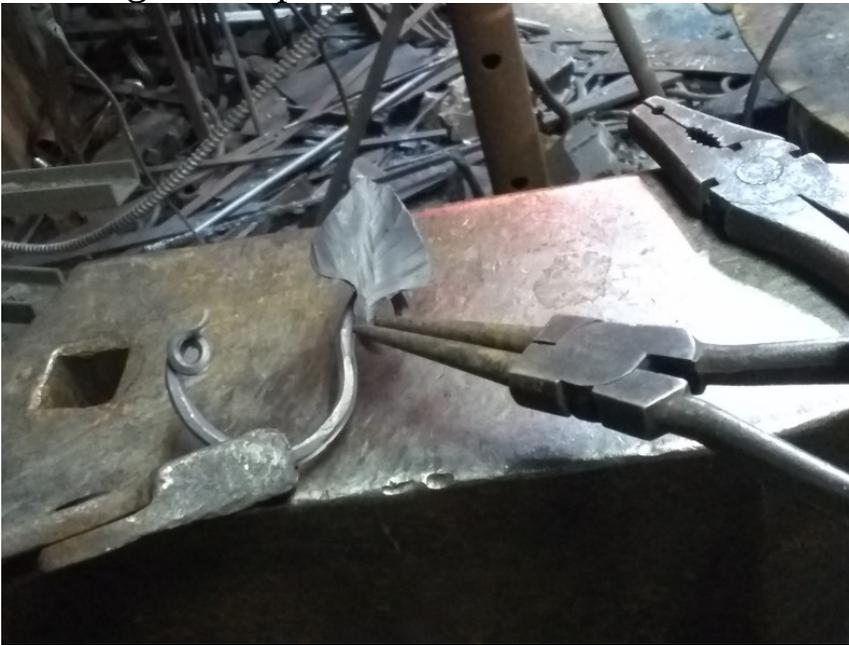
The brooch is shaped hot although photographed here cold. Use pliers that are round or that have the teeth sanded off. The copper is easily marked up with the teeth on steel tools.
