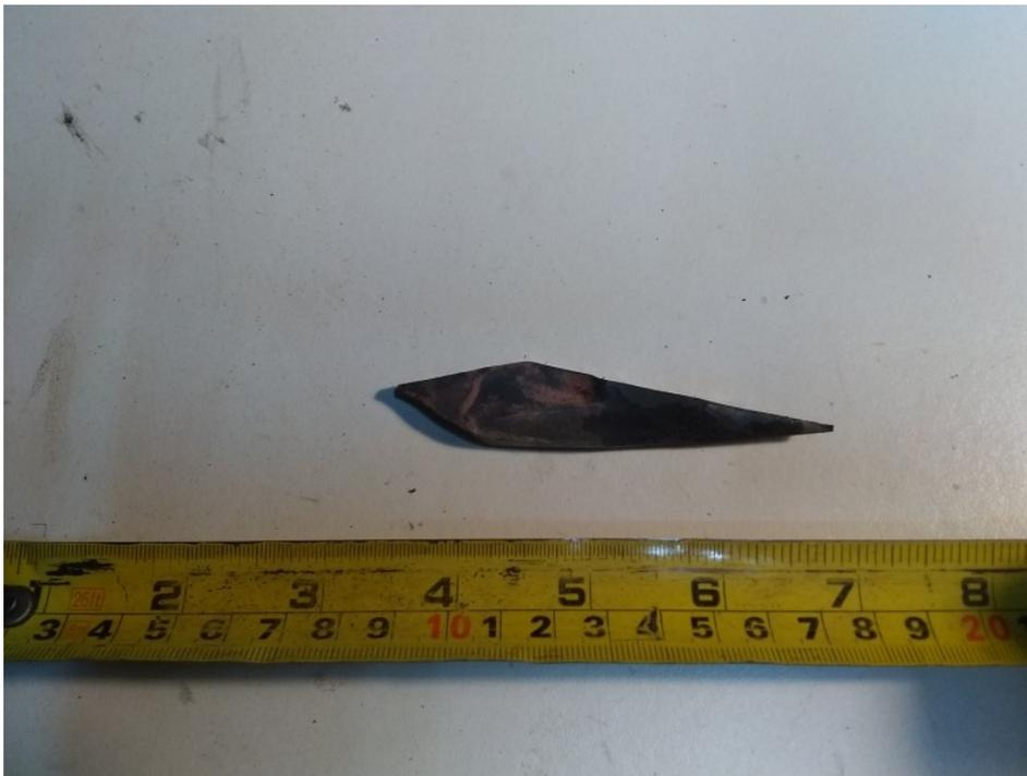
This photo shows the initial forging to create a basic shape that I can then turn into the leaf and the stem. Here I simply knocked the upper corner (in the above photo) down into the bar, then reworked the point to give the short taper.
