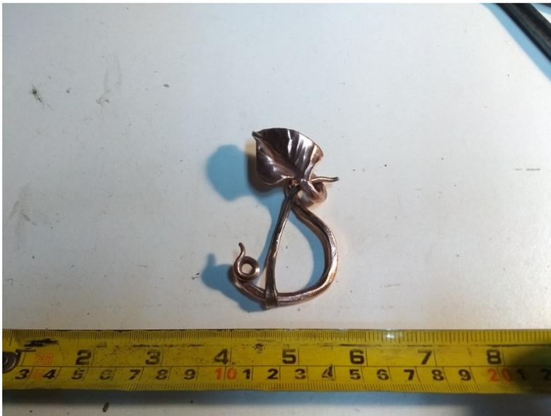
The final assembly is done cold. Make sure the pin is not too tight on the stem of the brooch. It should slide around easily.
