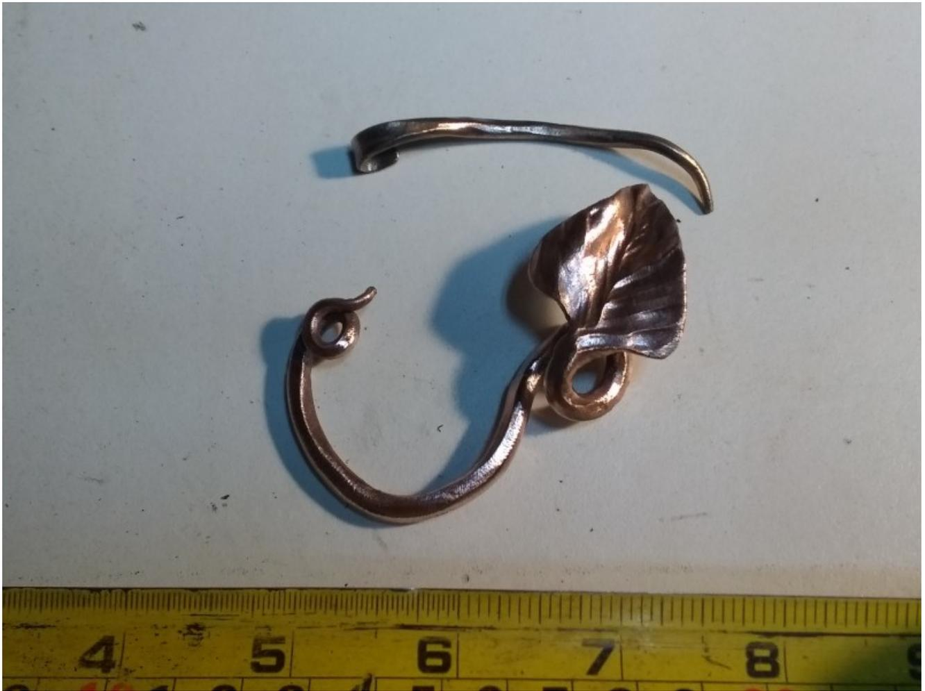
Above the pin has been forged out. This is also made out of copper and in this case is just a bit longer than 2 inches with the curl (which is still open in this photo). Both pieces have been buffed on the wire wheel to get rid of the thick oxide coating.
