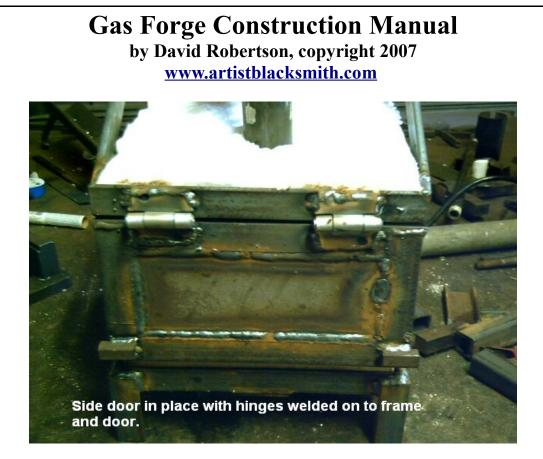
Make sure the hinges are straight because when things heat up any little twist is magnified and you may have a hard time opening the door.
