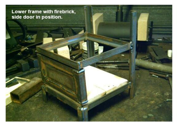
Remove door and weld the upper frame solidly to uprights.
