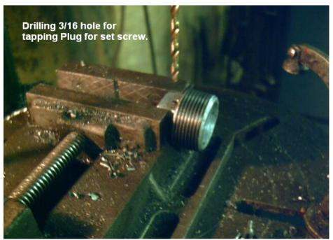
This is where you will thread using <sup>1</sup>/<sub>4</sub> inch tap for a set screw. This hole only needs to go through to the larger hole you drilled previously perpendicular to this one.
