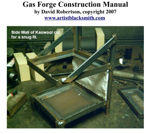
Now cut the Kaowool slightly larger than the top frame and fit in keeping it flat.
