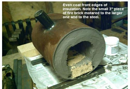
**Fire Brick Supports** The fire brick needs an arm on each side to support it.
