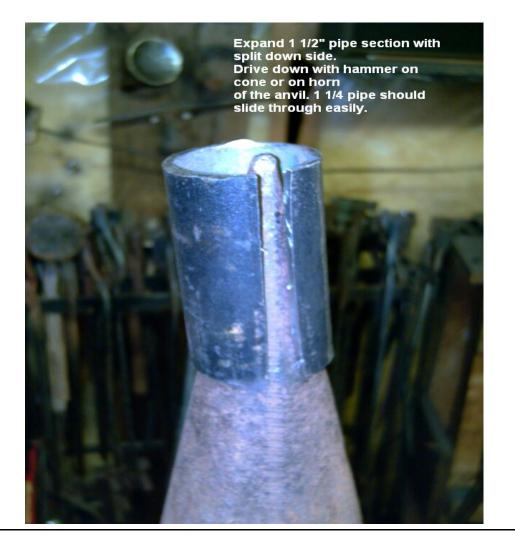
it easier. The important thing is to make it large enough that the 1 <sup>1</sup>/<sub>4</sub> pipe easily slides all the way through. It should not be sloppy but a smooth easy fit. This sleeve becomes the socket for the burner and is welded to the side wall of the forge.
