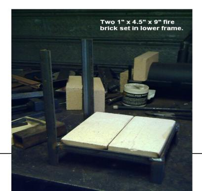
diagonal cut angle iron together for the floor. Two of the thin fire bricks should fit in with a little room to spare. I actually use the two thin fire bricks side by side on the welding table as a form for the angle iron frame so I know that they will fit in. It helps to keep it square as well. Weld in the floor sheet of steel. Weld on the short legs and the long legs as shown in the above picture.
