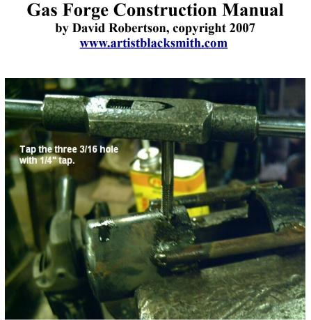
Tap the holes slowly with <sup>1</sup>/<sub>4</sub> inch tap. Remember <sup>1</sup>/<sub>2</sub> a turn reverse <sup>1</sup>/<sub>4</sub> turn to break off the cuttings, continue the next half turn. Make sure the tap is straight, use cutting oil. The other alternative is to drill <sup>1</sup>/<sub>4</sub> holes and weld nuts (with bolts threaded in them for alignment) to the out side of the pipe. I find the tapping looks cleaner. This is thin metal and taps quite easily.
