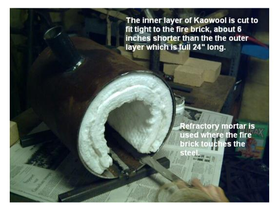
Once the fire bricks are set use a hacksaw blade to cut the Fibrofax from underneath the burner socket. I do this by gently forcing the blade through the insulation then slowly working the blade up and down cutting around the inside of the hole rubbing against the metal all the time. The hole you make should be slightly conic in shape with the large end of the cone being closest to the chamber. The 1  $\frac{1}{4}$  inch pipe should slide in with no trouble.
