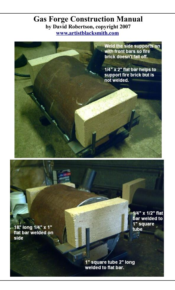
The  $\frac{1}{4}$  inch by 1 inch by 18 inch flat bars are the main side supports. These welded to the 1 inch square tubing 2 inches long and the  $\frac{1}{4}$  by  $\frac{1}{2}$  flat bar by 4 inches long make each side support. The welding process. Weld the ends of two of the square tube to the same side of the flat bar but at opposite ends. This should sit flat on the table. Weld the small flat bars vertical on the inner edge of the square tube. See the photo.
