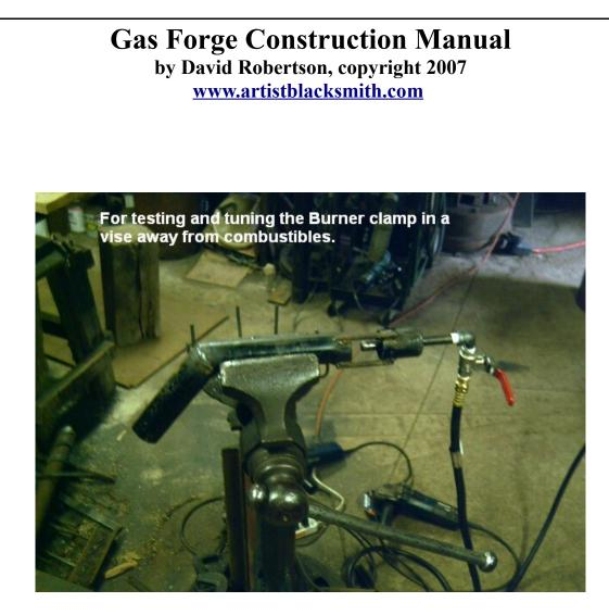
Once your flame is going release pressure on the set screws enough to slide the orifice in and out. Try moving back and forth and see how the flame changes. It is subtle. If you can find no change use the original  $\frac{1}{2}$  from end long burner tube position.
