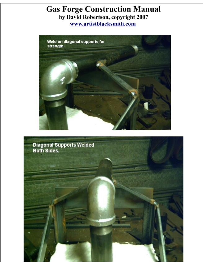
Diagonal supports on both sides of the burner tube for strength. If you ever need to do maintenance on the nozzle it simply just unscrews from the elbow. The fittings required for the blower and the orifice are seen in the picture below. The
