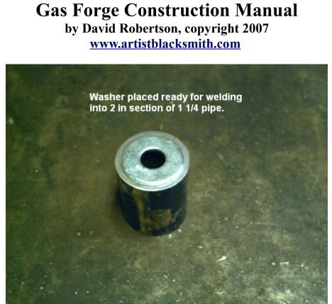
Next we set the  $\frac{1}{2}$  inch washer in the end of the 2 inch section of 1  $\frac{1}{4}$  inch pipe for welding. This becomes part of the alignment for the orifice. Weld the washer into the end of the pipe keeping it square.
