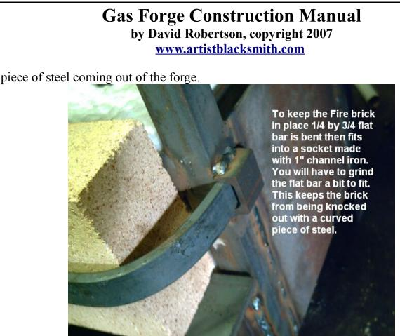
I actually bend this piece of  $\frac{1}{4} \times \frac{3}{4}$  flat bar in my forge over the anvil. You could do it cold or spot heat it with a torch. The end that fits into the  $\frac{1}{2} \times 1$  inch channel iron socket will need to be ground to fit. It should be easily removable.
