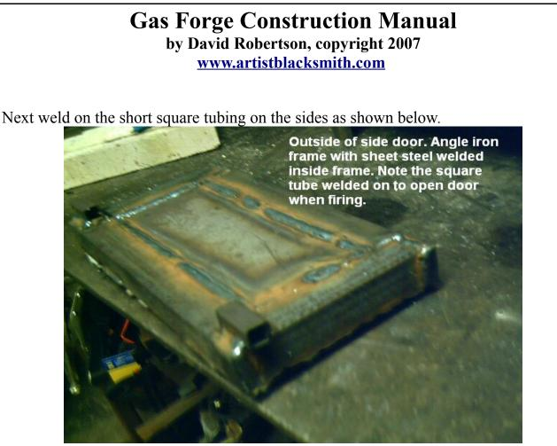
The idea behind this tube is that it gives you a place to put a square bar in while the forge is running to open the door if you have to put an odd shaped piece in for heating.
