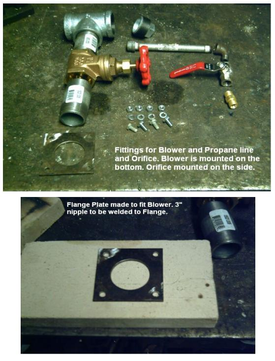
The flange plate is just 1/8 thick 3 x3 plate with a large hole cut into it and four small holes that match up holes in the blower flange. The key is to weld the threaded section of a 1  $\frac{1}{4}$  by 3 inch pipe nipple to the flange at the hole. This allows the flange to be screwed into the water gate valve giving an accurate way of controlling the air flow.
