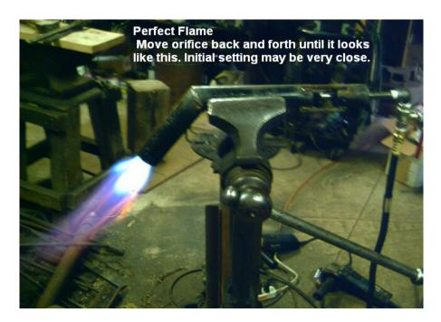
Once you get this shape and intensity of flame clamp your set screws down tight, but don't strip the threads. When tuning the burner you are looking for maximum blue flame with a minimum of yellow.
