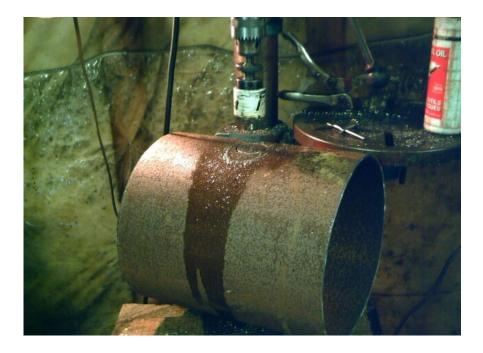
The hole cut through with the hole saw. This makes a clean cut that is easy to weld and has no slag to clean up after.
