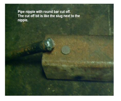
You should now have a capped pipe threaded on one end. The weld needs to be ground so that it will fit through the  $\frac{1}{2}$  inch washer.
