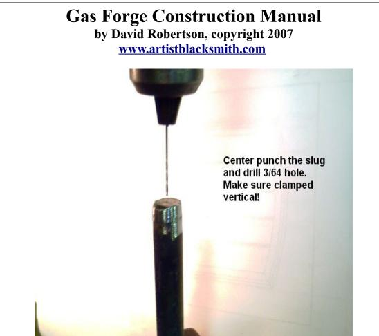
Use 3/64 drill bit. Center punch the hole and clamp in a drill press vertically and slowly drill the hole.
