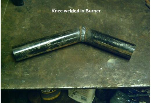
This knee construction creates a high degree of turbulence thoroughly mixing the propane and the air. This gives a more complete combustion and has an added advantage reducing the critical nature of the alignment of the orifice.
