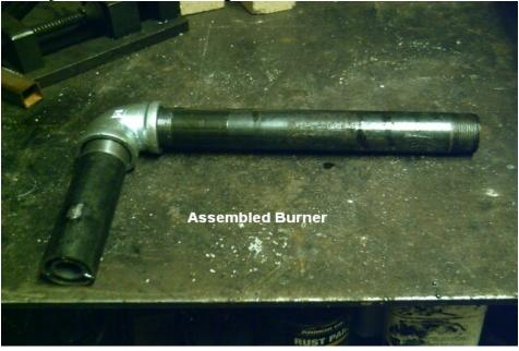
You do not need T-tape on any of the fittings a except propane. Take the assembled burner and place it in the hole so that the twelve inch piece rests on the back support. The burner should come straight down and be in the middle of the back support. The end of the nozzle should be <sup>3</sup>/<sub>4</sub> of an inch recessed from the inside of the chamber. (Protected by the Kaowool) Tack weld the horizontal pipe in position.
