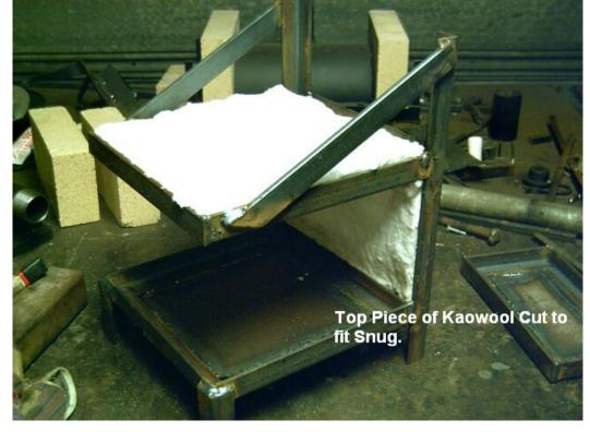
In the center of the top Kaowool you will need to cut a tight hole for the burner. I use a short piece of 1 <sup>1</sup>/<sub>4</sub> pipe and slowly rotate it back and forth as a circular cutter to wear a hole in the insulation. Keep you hand directly under it for support. Wear gloves and a mask. Discard the cut out.
