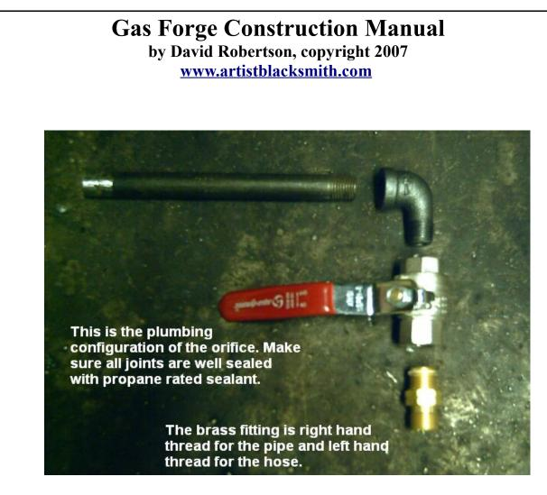
These are the components to make the orifice.
