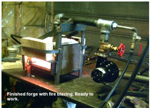
This forge is not as elegantly shaped as the previous forge and requires a great deal more cutting and welding of components to make it work. This forge is much more versatile and if you are able to weld well and don't mid piecing together little bits this forge will work very well for you. My primary production forge is the forerunner of this design.
