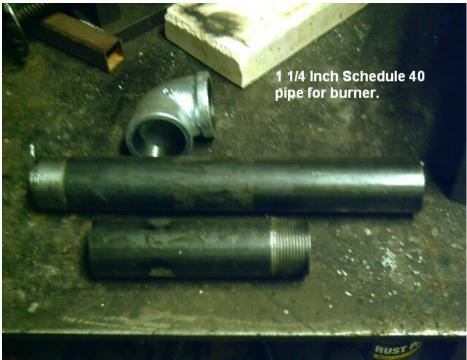
The long 1 <sup>1</sup>/<sub>4</sub> schedule 40 pipe 12" long needs to be threaded both ends, the 6 inch one
