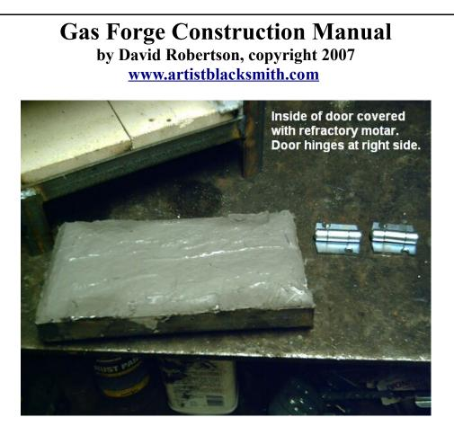
The above photo shows the inside of the door and the Kaowool coated with the refractory mortar. Follow the same procedure for drying and slow firing as in the pipe forge. You could also slow bake this in your oven or toaster oven at about 400 degrees for an hour to dry it out.
