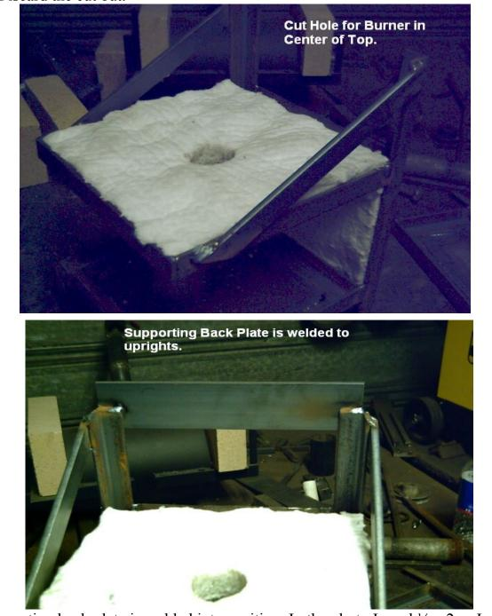
The supporting back plate is welded into position. In the photo I used  $\frac{1}{4} \times 2$  as I cut my
