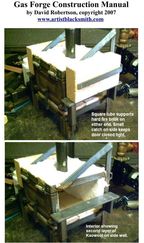
The distance between the floor of the forge to the bottom of the fire brick is 2 inches.
