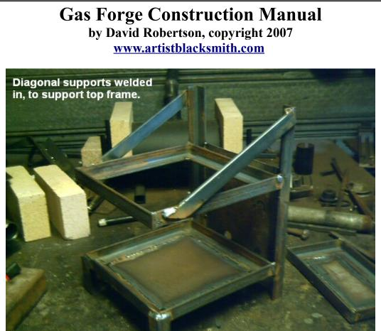
Once diagonals are in weld remaining sheet steel on to back of uprights.
