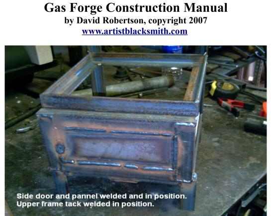
Clamp the upper frame to the tall vertical supports so that it rests  $\frac{1}{4}$  inch above the door resting on the fire brick. Use  $\frac{1}{4} \ge 1$  flat bar as a spacer. Make sure the top frame is level and tack weld into position.
