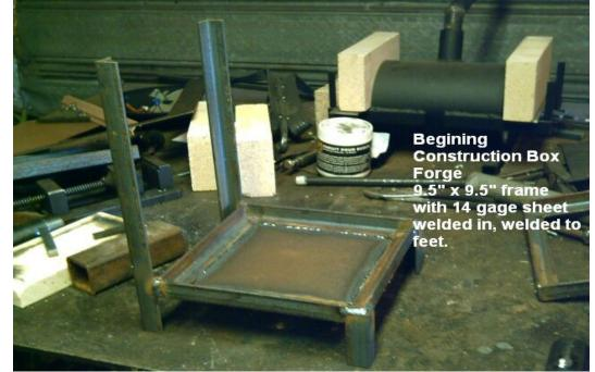
Make sure your supports are straight perpendicular. Start with welding 4 of the
